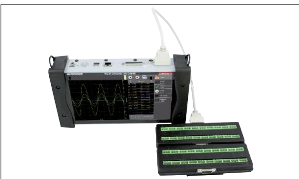
DAS240 equipped with 40 measurement channels
